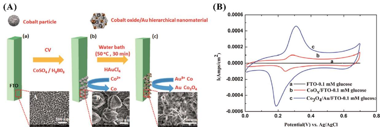
Fig. 5 (A) Shows the fabrication of Co<sub>3</sub>O<sub>4</sub>/Au hierarchically nanostructured electrode, and (B) presents cyclic voltammograms of the bare FTO, CoO<sub>x</sub>/FTO, and Au/Co<sub>3</sub>O<sub>4</sub>/FTO in 0.1 M NaOH solution with the presence of 0.1 mM glucose. Adapted with permission from ref. 112. Copyright © 2016 American Chemical Society.
