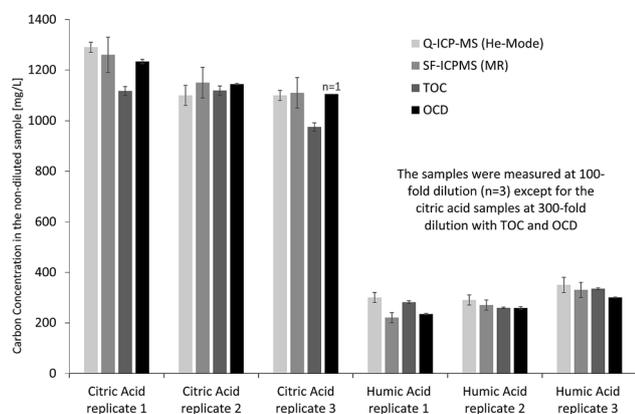
Fig. 2 Determination of total organic carbon in citric acid and humic acid model solutions by Q-ICP-MS, SF-ICP-MS, TOC and OCD.
