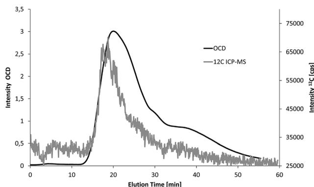
**Fig. 5** Overlay of fractograms of a soil extract recorded by FFF-Q-ICP-MS and FFF-OCD (the offset of 6 minutes between the fraction elution times from OCD and ICP-MS detection due to the larger internal volume of the OCD was determined by flow injection without FFF separation and subtracted from the elution time).
