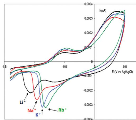
**Fig. 3** Cyclic voltammetry of PPy(1) membranes in aqueous alkaline chlorides: LiCl 0.1 M; NaCl 0.1 M; KCl 0.1 M; RbCl 0.1 M; CsCl 0.1 M. Scan rate of electrode potential 20 mV s<sup>-1</sup>.
