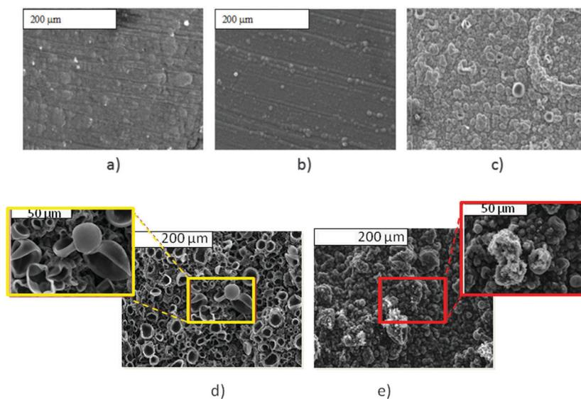
Fig. 6 S.E.M. studies of PPy films doped with different anions: (a) PPy(ClO<sub>4</sub>); (b) PPy(DBS); (c) PPy(**1**) and its surface modification by [NBu<sub>4</sub>]<sup>+</sup> and [PBU<sub>4</sub>]<sup>+</sup>, (d) and (e) respectively. (Fig. 6d reproduced with permission from ref. 8. Copyright 2002, John Wiley and Sons).
