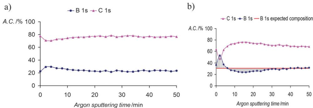
**Fig. 8** (a) XPS studies of PPy(7) membrane and (b) XPS studies of the overoxidized PPy(7) material. The membrane was set so that the side in contact with the solution is the first to be sputtered. (Reproduced with permission from ref. 10. Copyright 2005, Elsevier).
