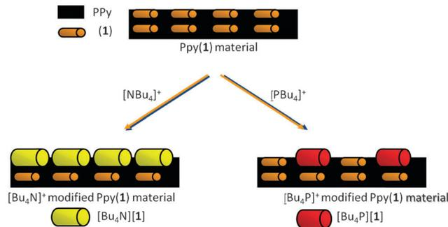
**Fig. 4** Graphical representation of the PPy(1) polymer modified by [NBu<sub>4</sub>]<sup>+</sup> and [PBu<sub>4</sub>]<sup>+</sup>.
