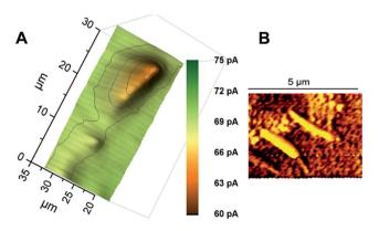
Fig. 2 (A) Negative feedback SECM image of individual AuNWs immobilized on a glass slide. The image was recorded with a 300 nm radius Pt probe at a potential of 0.3 V and a scan rate of 5  $\mu m\ s^{-1}$  in 1.5 mM ferrocenemethanol solution. (B) Representative AFM image of AuNWs immobilized on a glass slide.
