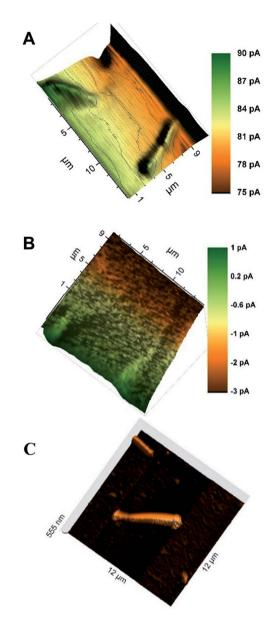
Fig. 7 SECM images of individual HRP-linked AuNWs immobilized on a gold-coated glass slide at (A) 0.3 V probe potential (positive feedback) and (B) 0 V probe potential after the addition of 0.3%  $\rm H_2O_2$  (SG/TC). The images were recorded with a 300 nm radius probe at a scan rate of 5  $\mu m~s^{-1}$  in 1.5 mM ferrocenemethanol solution in pH 6 SPB. (C) Representative AFM image of the same substrate.
