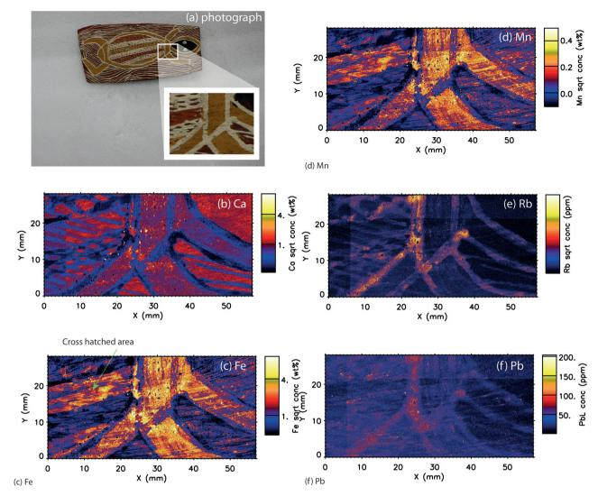
Fig. 5 (a) Visible light (photograph) of South Australian Museum object number A77584 – bark painting – indicating the approximately  $5 \times 3$  cm area that was analysed. Elemental maps are of this approximately  $5 \times 3$  cm analysed area. (b) Ca (c) Fe, (d) Mn (e) Rb (f) Pb.
