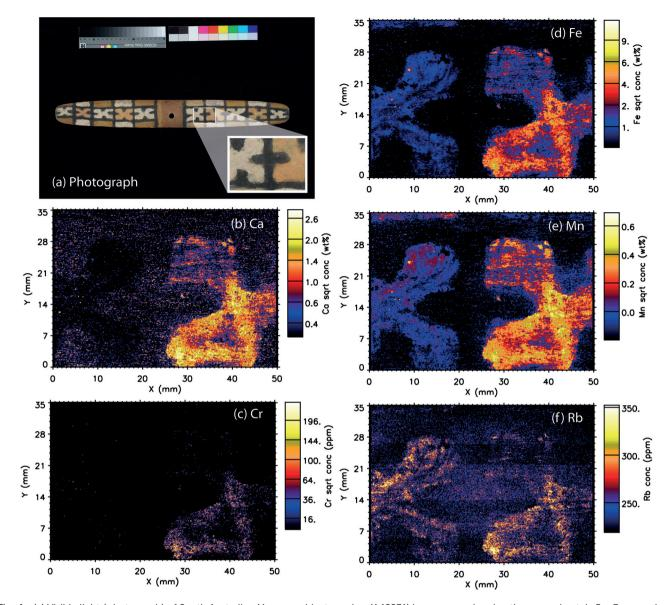
Fig. 4 (a) Visible light (photograph) of South Australian Museum object number (A42231) boomerang showing the approximately  $5 \times 3$  cm analysed area. Elemental maps correspond to this approximately  $5 \times 3$  cm analysed area. (b) Ca (c) Cr (d) Fe, (e) Mn (f) Rb. All images were flattened to the Compton image and displayed using the square root intensity scale.
