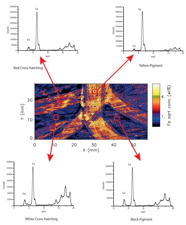
Fig. 3 Summed X-ray spectra from selected areas of the bark painting analysed in this study. Summed areas are approximately 4 mm diameter circles.
