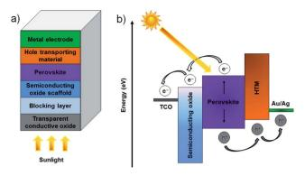
Fig. 2 (a) Structure and (b) operational mechanism of a typical PSC.
