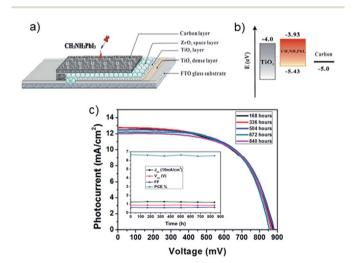
Fig. 4 (a) The structure of the first carbon counter electrode based PSC.64 (b) Energy level of TiO2, CH3NH3Pbl3 and carbon.64 (c) Current density-voltage curves of carbon cathode based PSCs over 840 hours. Inset: the effect of time on each value ( $J_{sc}$ ,  $V_{oc}$ , FF and PCE) of solar cell. Reprinted with permission from ref. 64 @ 2013, Nature Publishing Group.
