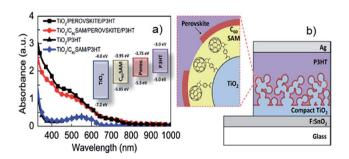
Fig. 7 (a) UV-vis spectra of P<sub>3</sub>HT and perovskite films with and without C<sub>60</sub>SAM. Inset: the energy level of the components used in Snaith's work.85 (b) The structure of the PSC fabricated with C<sub>60</sub>SAM layer between perovskite and TiO<sub>2</sub> layers. Reprinted with permission from ref. 85 © 2013, American Chemical Society.
