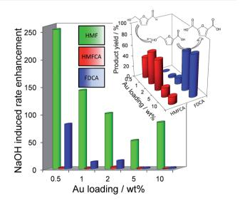
Fig. 4 (main) Impact of Au loading on the sensitivity of individual oxidation steps towards soluble base addition over Au/HT catalysts; (inset) Au loading dependent product selectivity in HMF oxidation in the absence of soluble base.
