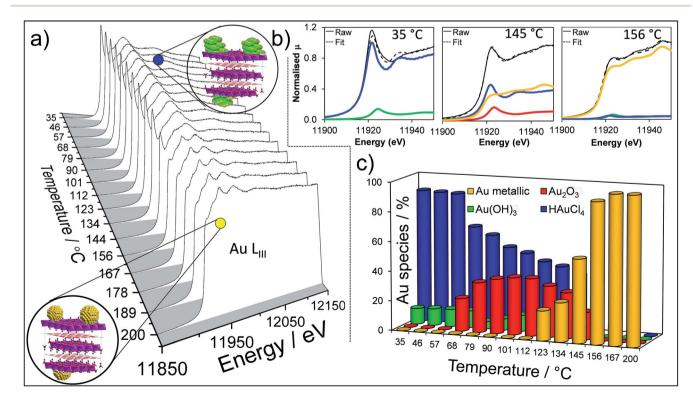
Fig. 1 In situ Au L<sub>III</sub> XANES during thermal processing of the HAuCl<sub>4</sub>/Mg-Al HT precursor: (a) thermal evolution of normalised XANES spectra; (b) representative least squares fitted XANES spectra to reference gold species; (c) quantitative thermal evolution of fitted Au species.
