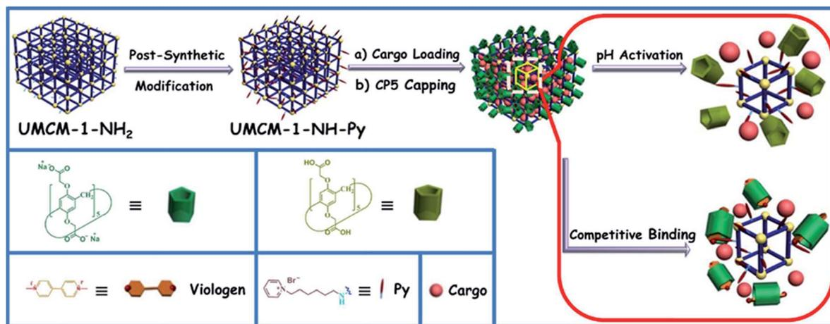
Fig. 1 Schematic representation of stimuli-responsive nanocarriers based on mechanized nanoMOFs (UMCM-1-NH<sub>2</sub>) with positively-charged pyridinium units (Py) as stalks encircled by pillarenes on the surfaces. The mechanized UMCM-1-NH<sub>2</sub> nanovalves can be operated either by pH changes or by competitive binding to regulate the release of cargo molecules, *i.e.*, rhodamine 6G (Rh6G) and doxorubicin hydrochloride (DOX).
