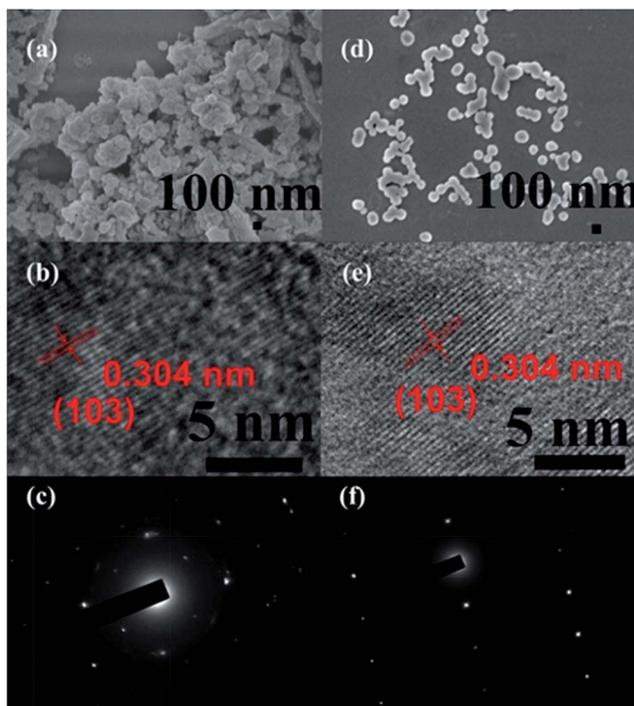
Fig. 2 (a) SEM image of UMCM-1-NH<sub>2</sub>, (b) HRTEM image of UMCM-1-NH<sub>2</sub>, (c) the corresponding electron diffraction pattern of UMCM-1-NH<sub>2</sub>, (d) SEM image of Rh6G-loaded, CP5-capped UMCM-1-NH-Py, (e) HRTEM image of Rh6G-loaded, CP5-capped UMCM-1-NH-Py, and (f) the corresponding electron diffraction pattern of Rh6G-loaded, CP5-capped UMCM-1-NH-Py.
