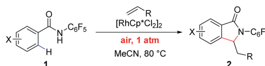
Scheme 1 Aerobic Rh(III)-catalyzed C–H olefination.
