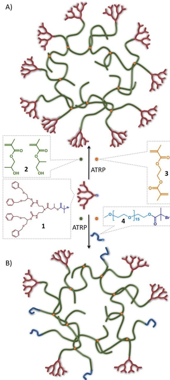
Fig. 1 Schematic representation of idealised hyp-polydendron synthesis. Atom transfer radical copolymerization (ATRP) of 2-hydroxypropyl methacrylate, **2**, and ethylene glycol dimethacrylate, **3**, initiated by the functional G<sub>2</sub> dendron, **1** to form (A) hyp-polydendrons; and (B) inclusion of a PEG<sub>16</sub>-initiator, **4**, to form hyp-polydendrons with controlled and mixed surface functionality.
