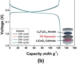
Fig. 5 Charge/discharge profiles of coin-type full cells as a function of cycle number, wherein the cells are cycled at a constant charge/discharge current density of 0.2 C (=0.40 mA cm $^{-2}$ )/0.2 C under a voltage range of 1.5–2.7 V: (a) LiCoO $_2$ /PC-CPE/Li $_4$ Ti $_5$ O $_{12}$ ; (b) LiCoO $_2$ /PE separator/Li $_4$ Ti $_5$ O $_{12}$ .
