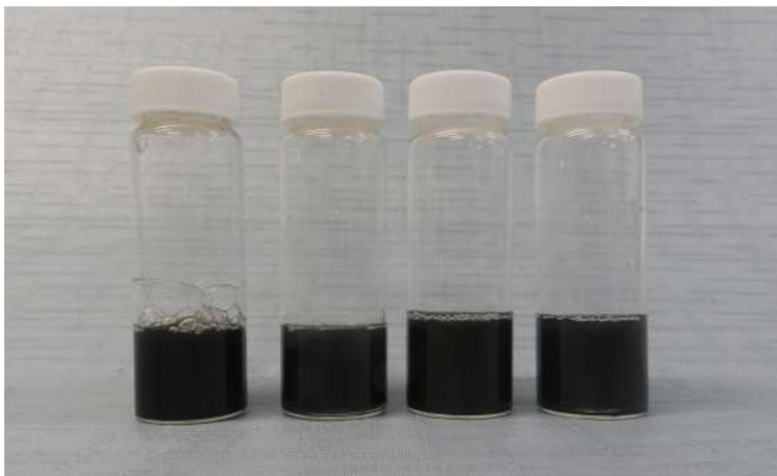
Figure 2: Digital images of EDoX-GO dispersed on aqueous solutions of SDS, SBDC, CATB, and TRITON X-100 (from left to right)
