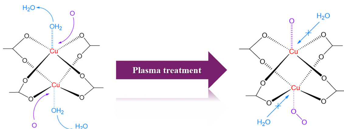
Fig. 7 Proposed \text{O}_2 plasma treatment mechanism of pore activation and protection. Reproduced from ref. 71 with permission from RSC, copyright 2017.
