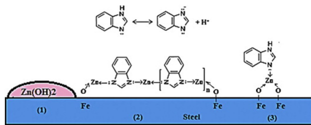
Fig. 12 Adsorption model of inhibitors released by Zn-MMT + BIA-MMT within artificial defects on steel surfaces. Reproduced with permission 120 from Elsevier.
