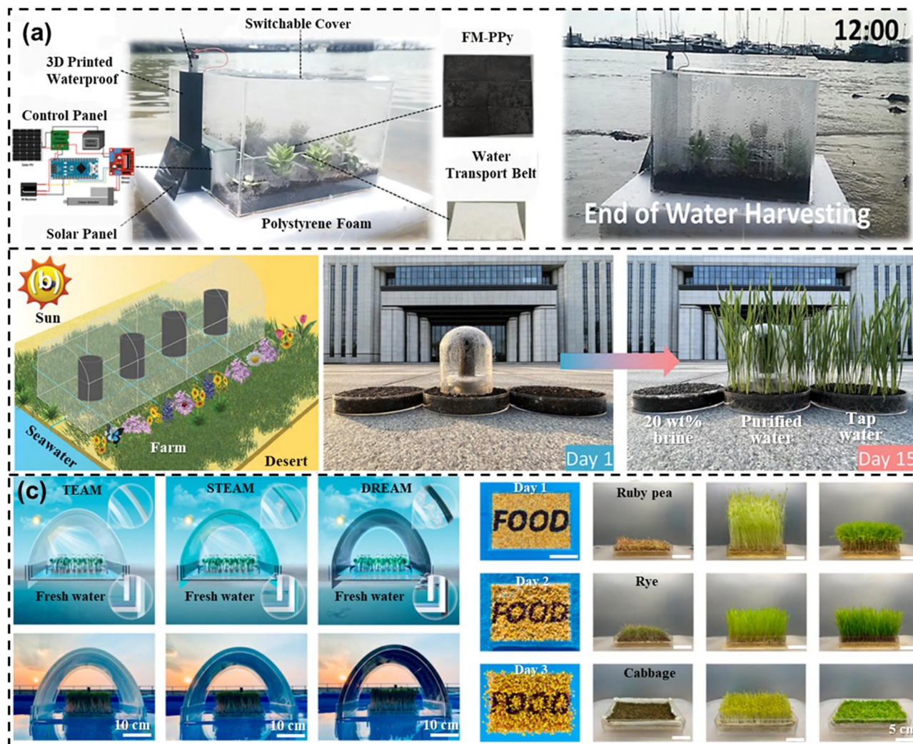
Fig. 27 ISVG-driven desalination for sustainable agricultural cultivation. (a) Image of an autonomous irrigation solar ocean farm. Reprinted with permission. Copyright 2022, Wiley-VCH; (b) schematic of potential applications of the continuous irrigation system. Reprinted with permission. Copyright 2024, Wiley-VCH; (c) the proof-of-concept about farming on the ocean (FOOD). Reprinted with permission. 210 Copyright 2023, American Chemical Society. TEAM represents the wood dome fabricated by a transparent evaporation material while STEAM and DREAM represent the wood dome fabricated by a semi-transparent evaporation material and dark evaporation material, respectively.
