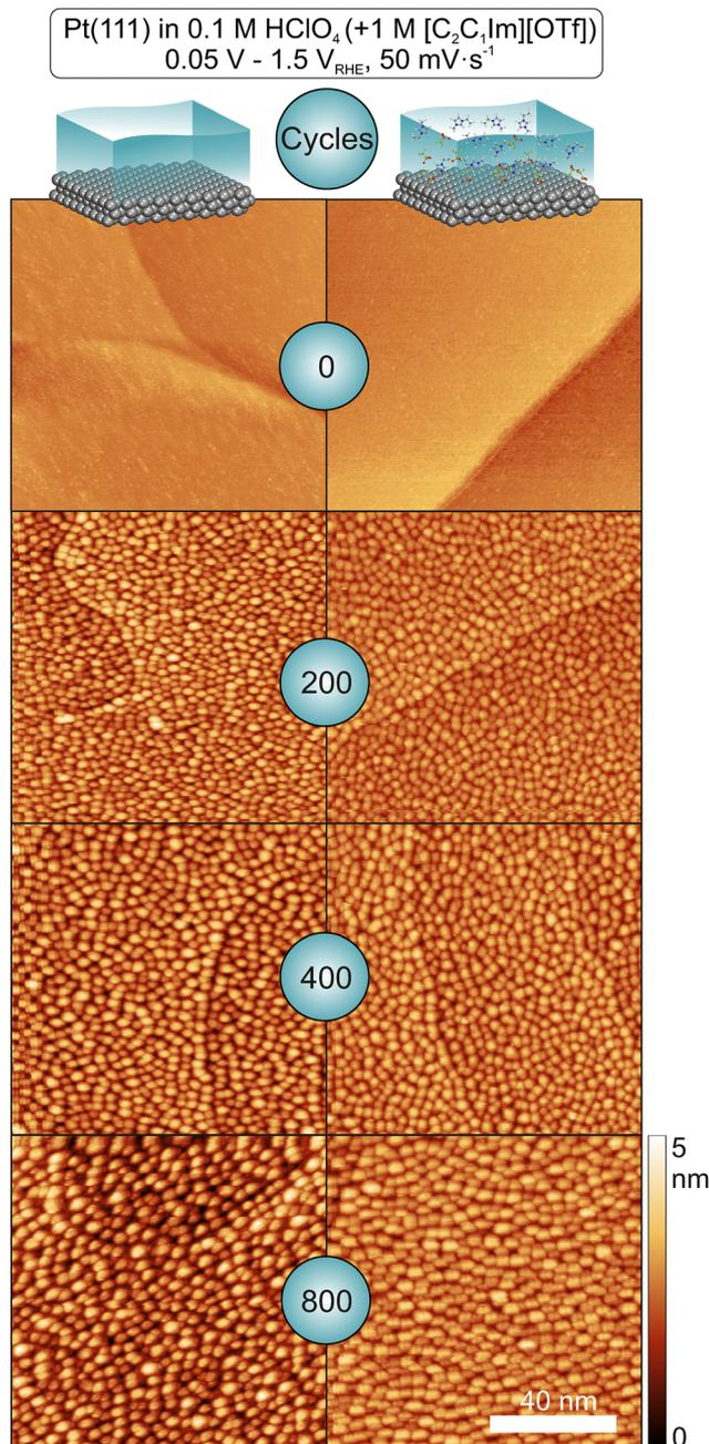
Fig. 5 EC-STM images ( $U_{\text{bias}}$  0.4 V,  $I_t$  0.2–1 nA) after extended ORCs (0.05–1.5  $V_{\text{RHE}}$ , 400  $\text{mV s}^{-1}$ ) in the absence (left) and presence (right) of 1 M  $[\text{C}_2\text{C}_1\text{Im}][\text{OTf}]$ . Supporting electrolyte was 0.1 M  $\text{HClO}_4$ .
