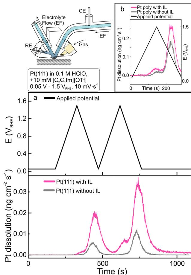
Fig. 3 (a) Online ICP-MS dissolution profiles for two consecutive CVs from Pt(111) in 0.1 M HClO<sub>4</sub> in the absence and presence of 10 mM [C<sub>2</sub>C<sub>1</sub>Im][OTf]. (b) Corresponding reference experiment of polycrystalline Pt. Applied electrochemical potential window 0.05–1.5 V<sub>RHE</sub>, scan rate 10 mV s<sup>-1</sup>.
