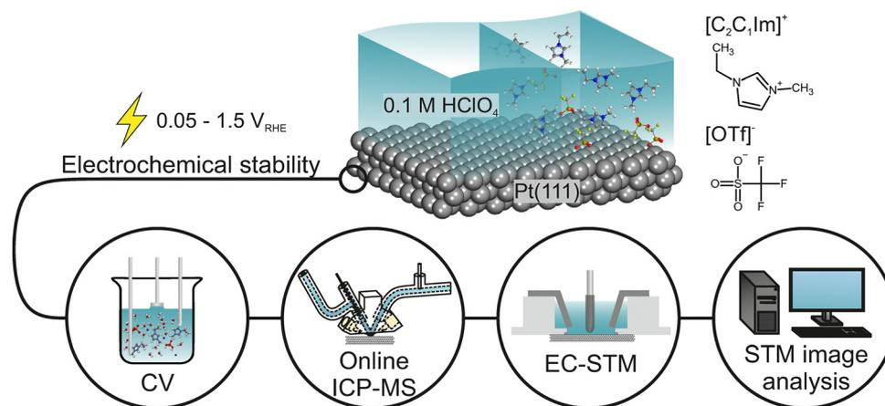
**Fig. 1** Electrochemical system studied in this work. Stability of Pt(111) in 0.1 M HClO<sub>4</sub> in absence and presence of the ionic liquid  $[\text{C}_2\text{C}_1\text{Im}][\text{OTf}]$ . We probe the electrochemical stability of the system applying CV, online ICP-MS, EC-STM and using an algorithmic pattern recognition approach to analyze STM images.
