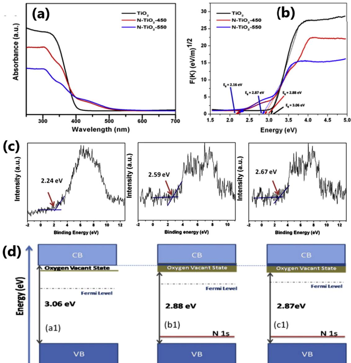
Fig. 7 (a) UV-vis absorbance spectra and (b) Tauc plot obtained from the reflectance spectra and (c) valence band edge analysis of  $\text{TiO}_2$ , N- $\text{TiO}_2$ -450, N- $\text{TiO}_2$ -550. (d) Proposed band diagrams of  $\text{TiO}_2$  and N-doped  $\text{TiO}_2$  catalysts. Reproduced with permission from ref. 115. Copyright©2016, Elsevier Ltd.
