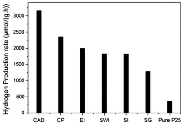
Fig. 17 Comparison of the photocatalytic hydrogen evolution rate on pure P25 and CuO/TiO<sub>2</sub> samples produced by different preparation methods, namely chemical adsorption decomposition (CAD), composite precipitation (CP), ethanol impregnation (EI), simple wet impregnation (SWI), stepwise impregnation (SI), and sol-gel (SG). Reproduced with permission from ref. 184. Copyright ©2014, Springer.
