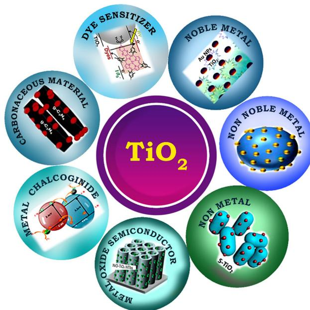
Fig. 3 Schematic representation of different types of chemical components used to improve the photocatalytic efficiency of TiO<sub>2</sub>.
