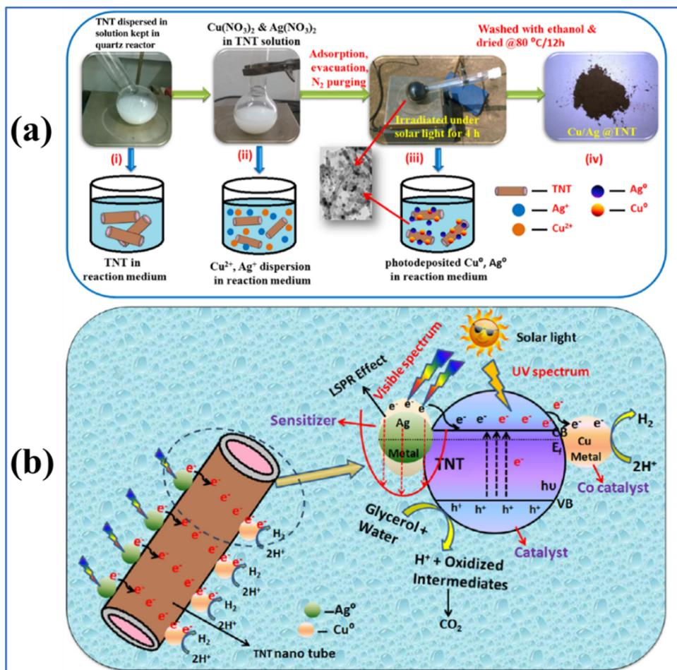
Fig. 6 (a) Schematic synthesis of Cu/Ag bimetallic deposition on titanium nanotubes (TNTs) and (b) charge separation and hydrogen evolution mechanism of as-synthesized Cu/Ag@TiO<sub>2</sub>. Reproduced with permission from ref. 99. Copyright©2017, Elsevier Ltd.
