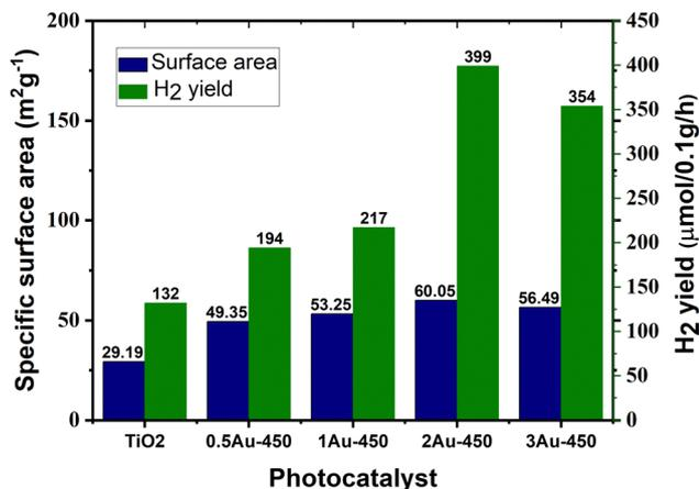
Fig. 19 Amount of hydrogen produced vs. surface area of photocatalyst for Au@TiO<sub>2</sub>:0.5Au-450, 1Au-450, 2Au-450 and 3A-450 under natural solar light. Adopted from ref. 166. Copyright ©2018, the Royal Society of Chemistry.
