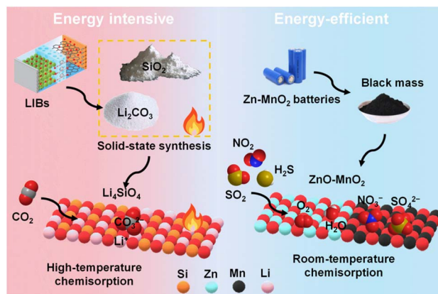
Fig. 6 An illustration showing energy-intensive and energy-efficient upcycling of battery waste for acidic gas removal.
