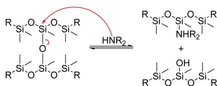
Fig. 16 Cleavage of Si–O bond by an amine.
