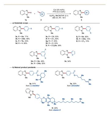
Scheme 2 Substrate scope for aryl iodides in photo-induced copper(I)-catalyzed C-H arylations at room temperature.
