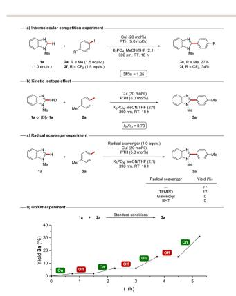
Scheme 5 Key mechanistic experiments.
