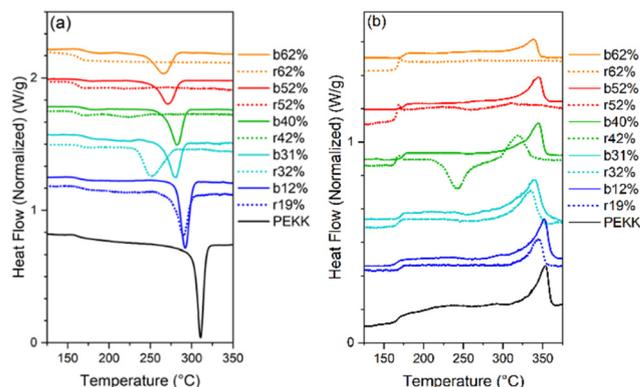
Fig. 7 Standard DSC scans of blocky (solid lines) and random (dashed lines) BrPEKK (a) first cool after removal of thermal history and (b) second heat. All DSC scans were performed at  $10 \text{ °C min}^{-1}$  in a nitrogen atmosphere.
