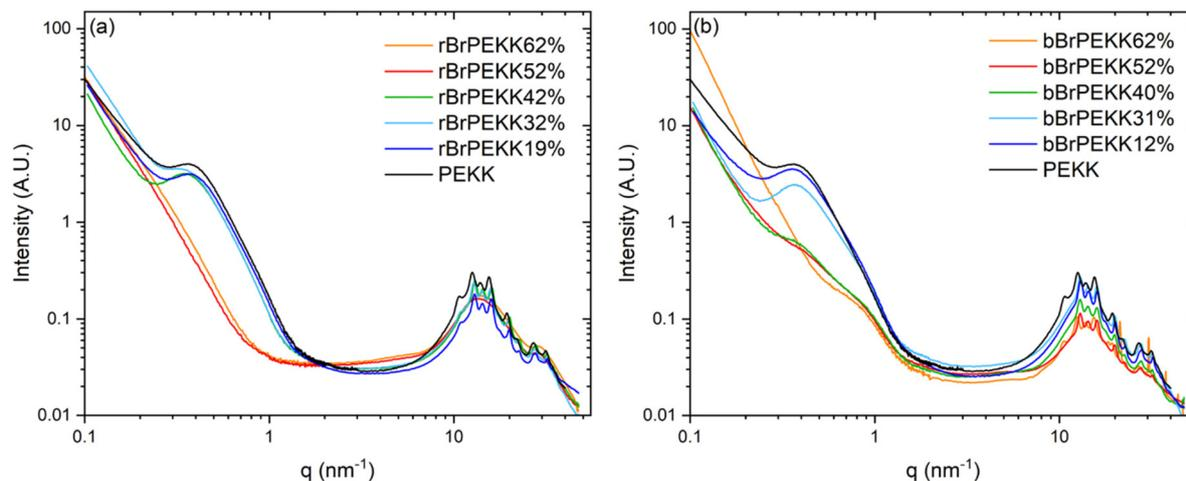
**Fig. 11** Small, mid, and wide-angle X-ray scattering profiles of (a) random BrPEKK and (b) blocky BrPEKK. All samples were isothermally crystallized from the melt at 280 °C for 30 minutes in a nitrogen atmosphere.
