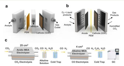
Fig. 7 Application of the acidic CO<sub>2</sub>RR in a tandem electrolyzer system for achieving high SPCE. Schematics of the (a) flow cell and (b) MEA. (c) Zero carbon loss tandem MEA system for MEA to MEA, CO<sub>2</sub> to CO, and CO to C<sub>2</sub>H<sub>4</sub>. A Reproduced with permission from ref. 47. Copyright 2023, The Royal Chemical Society.
