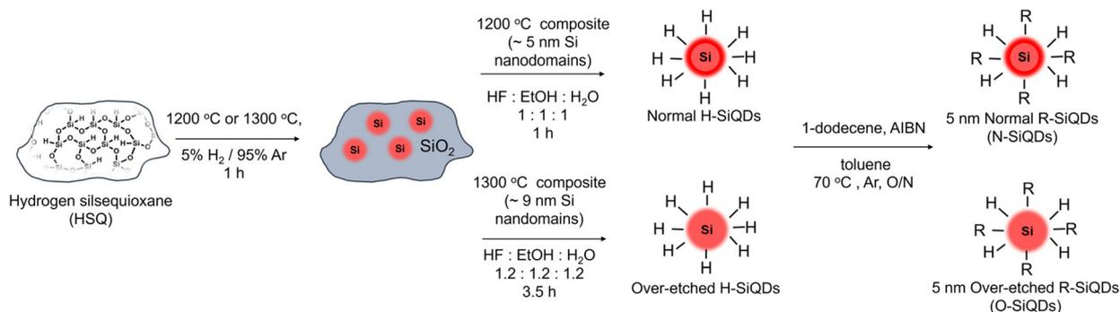
**Scheme 1** Preparation of 'normal' and 'over-etched' dodecyl-functionalized SiQDs. Freestanding H-SiQDs were liberated from HF-etching of thermally-processed HSQ, followed by radical-initiated hydrosilylation with 1-dodecene.
