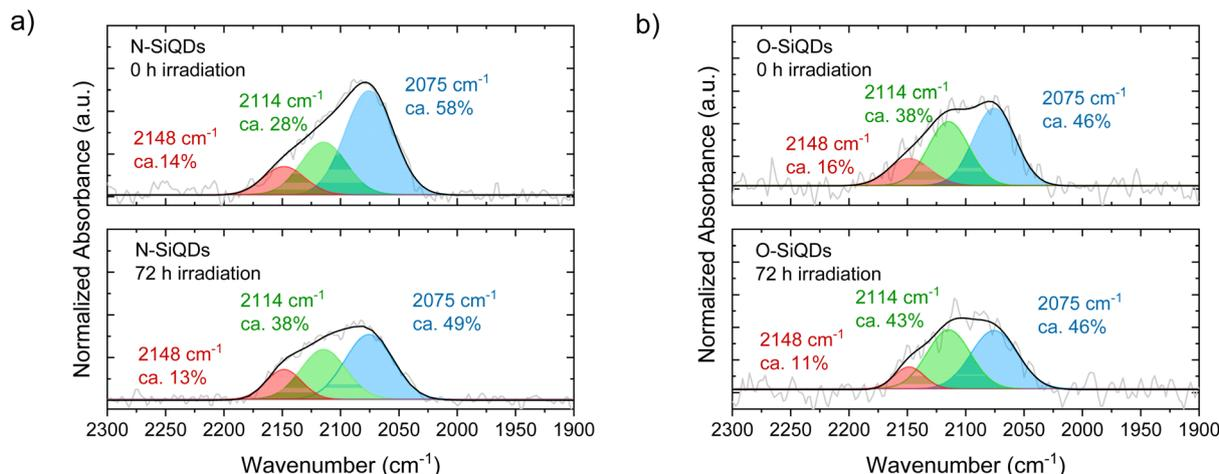
**Fig. 4** Deconvoluted FT-IR spectra of (a) N-SiQDs and (b) O-SiQDs as prepared (top) and following 72 h UV irradiation (bottom) spanning the SiH<sub>x</sub> stretching region and deconvoluted to show the contributions from SiH<sub>3</sub> (red), SiH<sub>2</sub> (green), and SiH (blue) components. In general, a decrease in the SiH<sub>3</sub> contribution is noted after irradiation.
