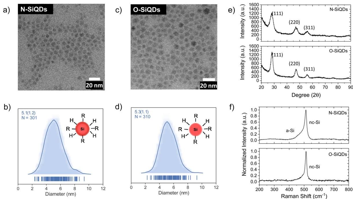
**Fig. 1** Structural characterization of the SiQDs used in this study. Brightfield TEM images show equivalent physical dimensions of (a) N-SiQDs ( $5.1 \pm 1.2$  nm) and (c) O-SiQDs ( $5.3 \pm 1.1$  nm). The respective size distributions, (b) and (d), are presented as average-shifted histograms. (e) XRD patterns, and (f) Raman spectra show evidence of greater long-range order in O-SiQDs.
