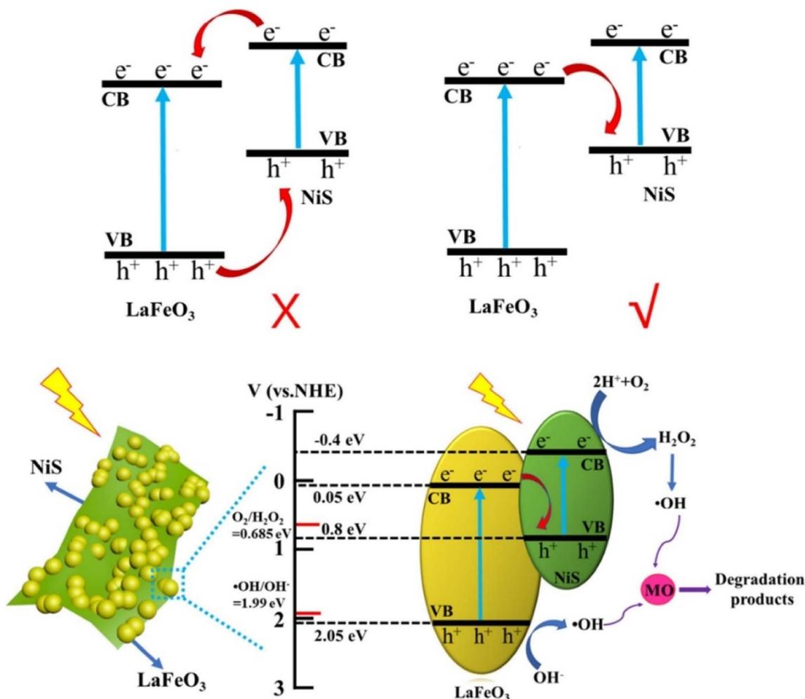
Fig. 1 Schematic diagram showing how NIS/LFO heterostructures photocatalytically degrade MO.<sup>12</sup>
