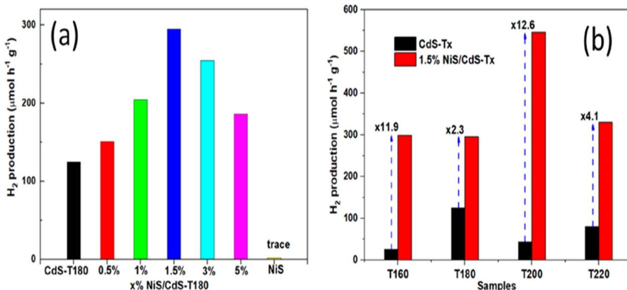
Fig. 13 (a) The photocatalytic efficacy of CdS-T180 with varying concentrations of NiS (b) photocatalytic activity of CdS-T<sub>x</sub> samples before and after the addition of 1.5 wt% NiS for H<sub>2</sub> production.<sup>58</sup>
