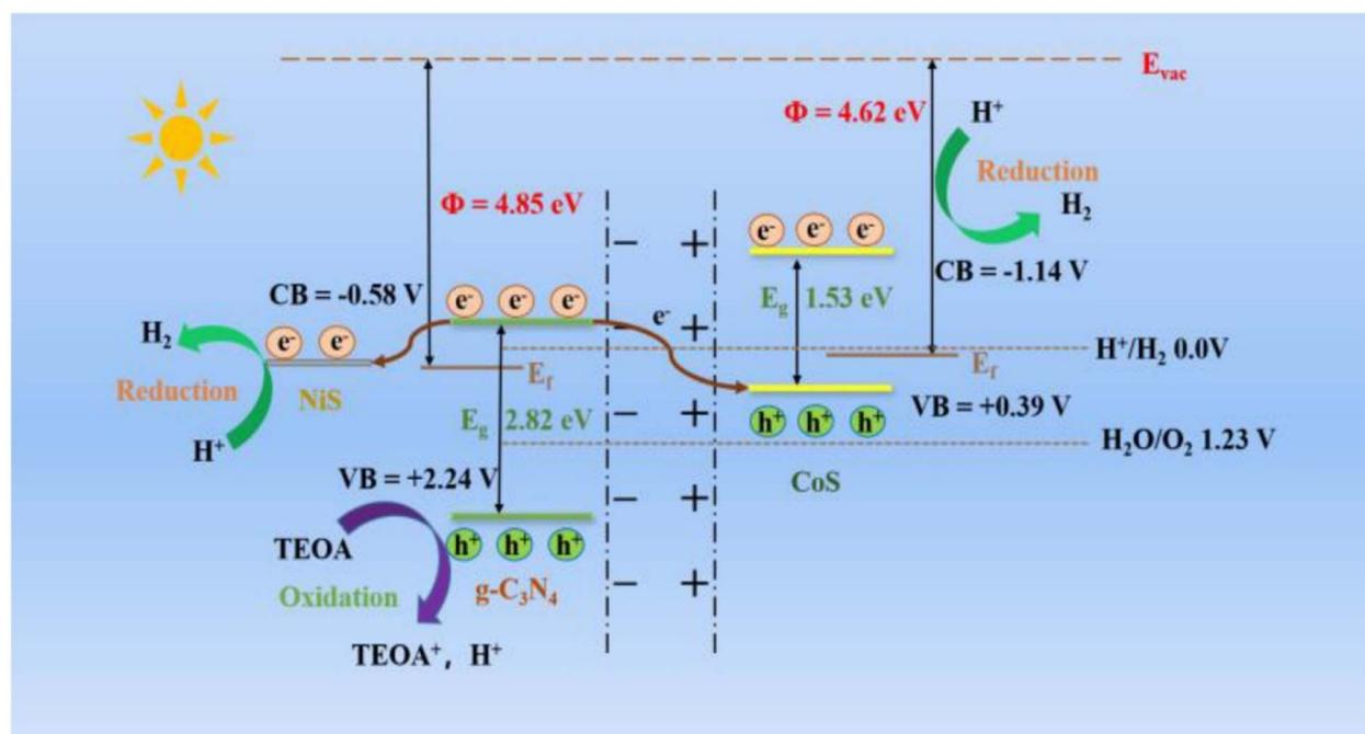
Fig. 16 The band structure and hydrogen evolution mechanism of CoS/CN/NiS composites are under consideration.<sup>67</sup>
