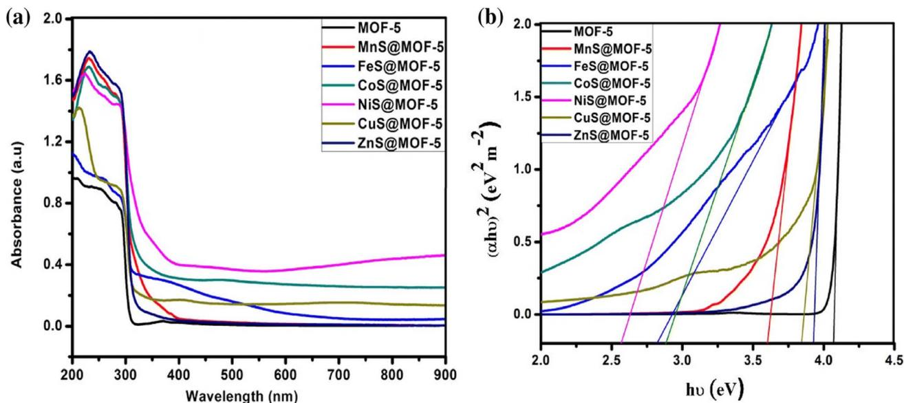
Fig. 15 (a) UV-vis spectrum (b) Tauc plot of bare MOF-5 and TMS@MO5.<sup>65</sup>
