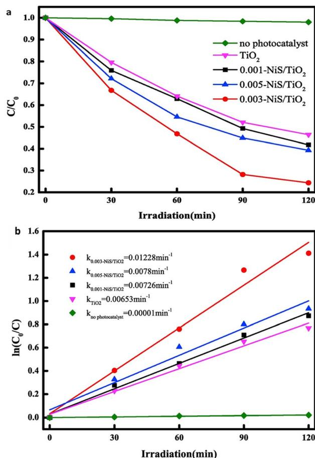
Fig. 12 (a) The degradation rates for photocatalysis and (b) the kinetic curves of methylene orange (MO) degradation for both pure TiO<sub>2</sub> nanosheets arrays (NSAs) and  $x$ -NiS/TiO<sub>2</sub> p-n heterostructured NSAs with varying NiS content.<sup>53</sup>
