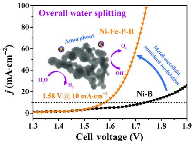
Fig. 10 The overall water-splitting performance of Ni-Fe-P-B@CFP.<sup>47</sup>
