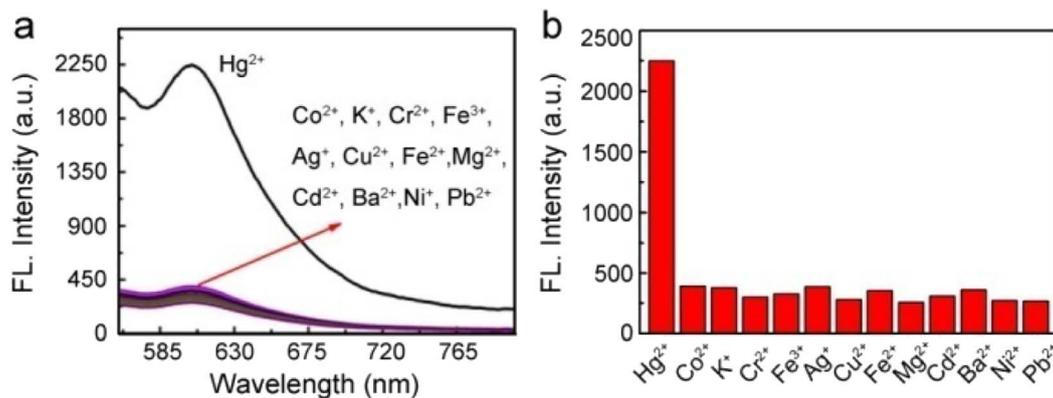
Fig. 4 (a) Fluorescence spectra for the fluorophore-labeled Au@SiO<sub>2</sub> probe in the presence of 1.0 equivalent of Hg<sup>2+</sup>, Co<sup>2+</sup>, Fe<sup>3+</sup>, Cd<sup>2+</sup>, Fe<sup>2+</sup>, K<sup>+</sup>, Cr<sup>2+</sup>, Cu<sup>2+</sup>, Pb<sup>2+</sup>, Mg<sup>2+</sup>, Ag<sup>+</sup>, Ba<sup>2+</sup>, and Ni<sup>2+</sup>. The final concentration of the probe and metal ions are all 0.5 μM. (b) Selectivity of NP sensors plotted in histogram form.
