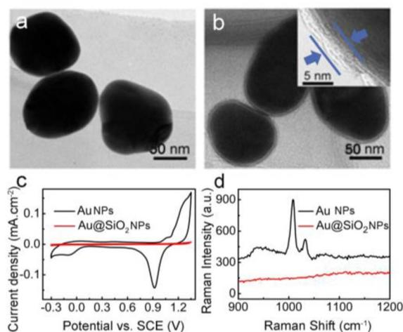
**Fig. 1** TEM images for the (a) 80 nm Au NPs and (b) corresponding Au@SiO<sub>2</sub> NPs with an external 4–5 nm SiO<sub>2</sub> shell. Inset is a TEM image of Ag@SiO<sub>2</sub> NPs to show the silica shell. (c) Cyclic voltammograms of Au NPs and Au@SiO<sub>2</sub> in 0.5 M H<sub>2</sub>SO<sub>4</sub> solution, scan rate: 0.1 V s<sup>-1</sup>. (d) Raman spectrum of pyridine; 0.001 M pyridine on Au and Au@SiO<sub>2</sub> on a Si wafer, respectively.
