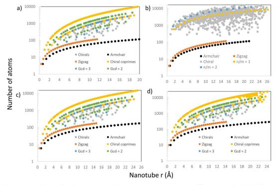
Fig. 6 Plots of the number of atoms for all chiral and achiral nanotubes in the range n, m < 30 vs. their radius for 4 different materials: (a) SWCNTs, (b) PNTs, (c)  $MoS_2$  NTs and (d)  $Ti_3C_2$  NTs. In a, c, and d, those NTs with n, m pairs which are coprime are highlighted in yellow, those with g.c.d = 2 in green, and those with g.c.d = 3 in blue. For b, the series of NTs with n/m = 1 and n/m = 2 are highlighted in yellow and blue, respectively
