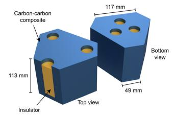
**Fig. 4** The schematic diagram of the six-sided polygon-shaped RHS is depicted, where the yellow and blue areas indicate the insulating container for the radioisotope and the carbon composite material, respectively. This figure is redrawn by the authors based on the original figure.<sup>8</sup>
