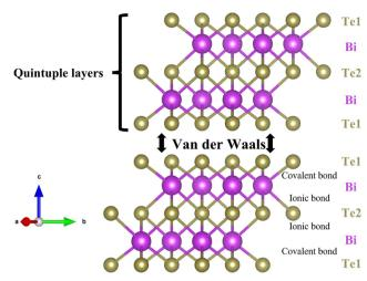
Fig. 10 Bi<sub>2</sub>Te<sub>3</sub> exhibits a rhombohedral structure consisting of guintuple layers, Te1-Bi-Te2-Bi-Te1, connected by van der Waals bonding along the c-axis. Information on the crystal structure was sourced from materialproject.org and visually represented using VESTA.48
