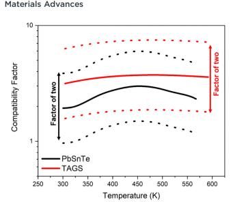
Fig. 9 The compatibility factors of TAGS<sup>37</sup> and PbSnTe<sup>47</sup> in the p-type legs of the multi-mission radioisotope thermoelectric generator (MMRTG). The bold and dotted lines represent the compatibility factors calculated based on egn (3) and the compatible range of a factor of two, respectively.
