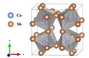
Fig. 11 Illustration of the crystal structure of the  $CoSb_3$ -based alloy, which crystallizes into octahedrons within the space group  $Im\bar{3}$ . The structure is characterized by a void at the center of the cubic lattice. Crystal structure information was sourced from materialproject.org and visually represented using VESTA.<sup>48</sup>
