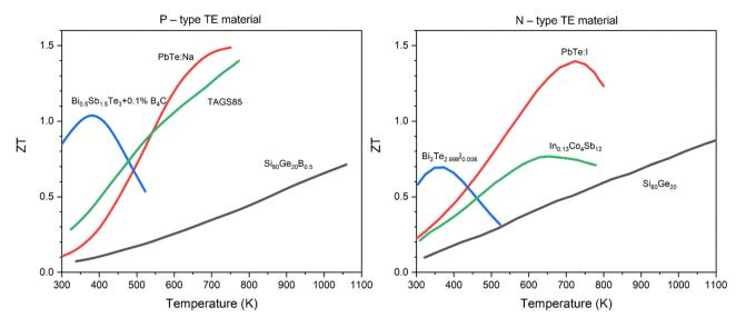
Fig. 7 Relationships between zT and optimal operating temperature ranges for selected TE materials. On the left-hand side, p-type materials include Bdoped SiGe, <sup>31</sup> PbTe:Na, <sup>30</sup> Bi<sub>0.5</sub>Sn<sub>1.5</sub>Te<sub>3</sub> +  $0.1B_4$ C, <sup>36</sup> and TAGS85. <sup>37</sup> On the right-hand side, n-type materials feature SiGe, <sup>38</sup> PbTe:I, <sup>32</sup> Bi<sub>2</sub>Te<sub>2.992</sub>I<sub>0.008</sub>, <sup>35</sup> Infilled CoSb<sub>3</sub>. 39,40
