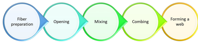
Fig. 3 Steps involved in the formation of nonwovens.
