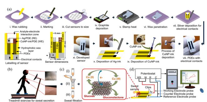
Fig. 5 (a) Schematic of the design and manufacture of two-electrode enzyme-free human sweat glucose sensor (i-ix) with the sensor dimensions and labelling, (b) secretion of sweat during treadmill exercise at room temperature, (c) filtration of sweat, and (d) set-up for developed sensor connected to a potentiostat with a computer system for detecting the level of sweat glucose in a human sweat sample. Reproduced with permission from ref. 150 Copyright 2022, Elsevier.
