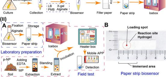
Fig. 8 (I) Schematic illustration of manufacturing of paper-strip biosensor. (II) Diagram of whole-cell biosensor device for detecting MP and pnitrophenol (p-NP): flow-diagram of the fabrication and utilization (A) and objective drawing (B) of whole-cell paper-strip biosensor. Reproduced with permission from ref. 172 Copyright 2023, Elsevier.
