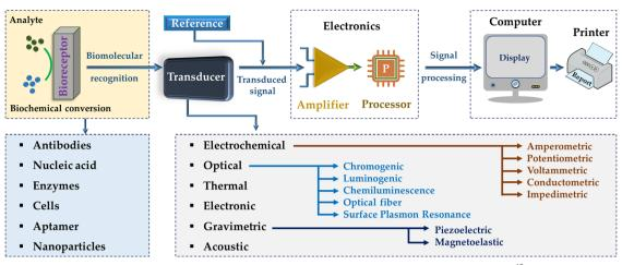
Fig. 1 Schematic illustration of a biosensing device, which is comprised of a bioreceptor, transducer, and amplifier.<sup>42</sup>
