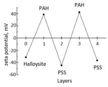
**Fig. 2** Synthesis nanocarriers from halloysite loaded with 2-mercaptobenzothiazole. Zeta potential during polyelectrolyte deposition on halloysite nanotubes at pH 7.5. Reproduced from ref. 101 with permission of publisher. Copyright 2008 American Chemical Society.
