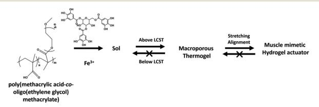
Fig. 7 Schematic representation of the design of hydrogel actuators based on a combination of thermoinduced phase separation and mechanical alignment.
