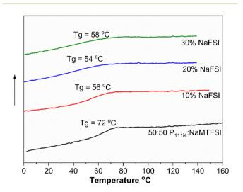
Fig. 4 DSC plot of 50:50 mol% polymer blends and the addition of NaFSI salt in wt% at 10 K min<sup>-1</sup>.
