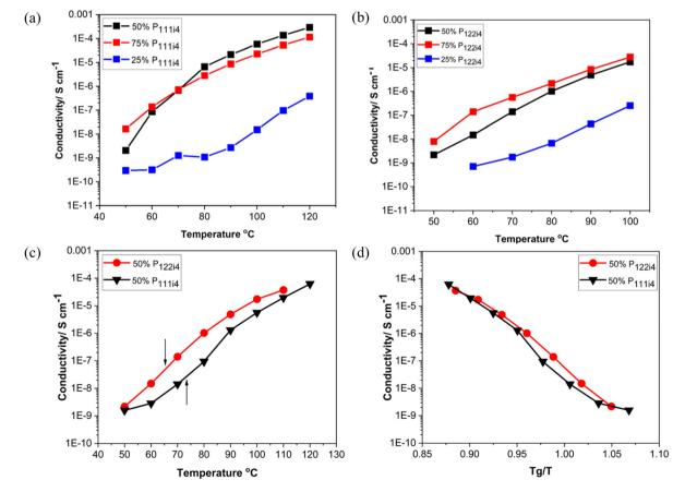
Fig. 2 Ionic conductivity at different concentrations of poly-NaMTFSI with (a) poly-P<sub>11114</sub>MTFSI and (b) poly-P<sub>12214</sub>MTFSI, (c) ionic conductivity of 50 mol% polymer blends of the mixed co-cation of poly-P<sub>111i4</sub> and poly-P<sub>122i4</sub> with poly-NaMTFSI. (d) Ionic conductivity as a function of the bulky cation with inverse temperature normalized by  $T_{\rm g}$  for each polymer blend.
