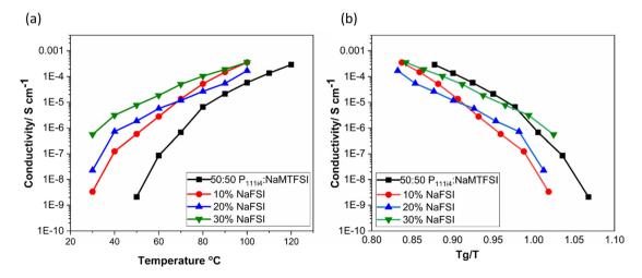
Fig. 5 (a) Ionic conductivity of 50:50 mol% polymer blends and the addition of NaFSI salt in wt% at an elevated temperature and (b) ionic conductivity as a function of NaFSI salt concentration with inverse temperature normalized by  $T_{\rm g}$  for each polymer blend.
