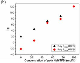
Fig. 1 (a) DSC thermograms of neat poly-NaMTFSI and 50 mol% poly- $P_{111i4}$ MTFSI and poly- $P_{122i4}$ MTFSI polymer blends. (b)  $T_g$  of different polymer blends with poly-NaMTFSI with both poly- $P_{111i4}$ MTFSI and  $P_{122i4}$ MTFSI at different compositions. Scan rate: 10 K min<sup>-1</sup>.
