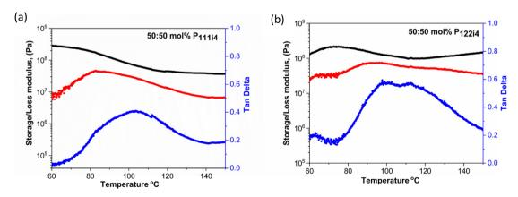
Fig. 3 Storage modulus (E', black), loss modulus (E'', red) and  $\tan \delta$  (blue) as a function of temperature for the 50 mol% polymer blends of the mixed co-cation of poly-NaMTFSI with (a)  $P_{111i4}MTFSI$  and (b)  $P_{122i4}MTFSI$ .
