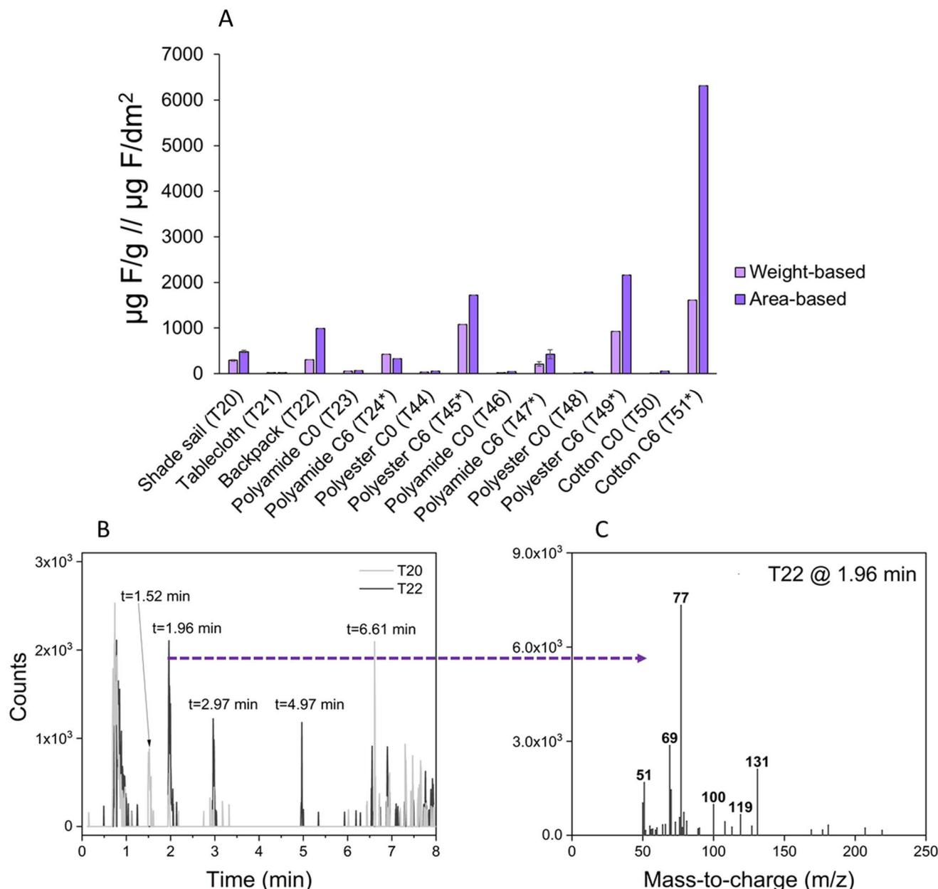
**Fig. 6** (A) Total fluorine concentrations in textiles based on weight (light purple) and area (dark purple). (B) Extracted ion chromatogram ( $m/z$  131) of the shade sail textile (T20) and the backpack (T22) where the presence of PFAS was initially unknown with the specific eluting retention times (1.96, 2.97 and 4.97 min). (C) The corresponding mass spectra containing typical  $m/z$  peaks suggest that T22 contains a C8-SFP. Error bars represent standard deviation.
