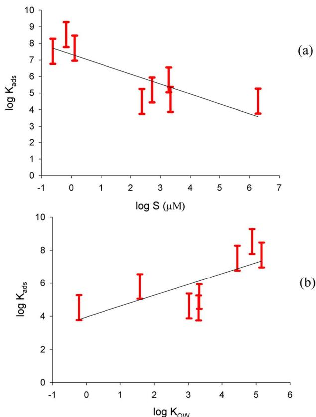
Fig. 4 Plots of  $\log K_{\text{ads}}$  as determined here against (a)  $\log S$ , with the solubility expressed in  $\mu\text{mol L}^{-1}$ ; (b)  $\log K_{\text{OW}}$ . The red bars indicate the range of  $\log K_{\text{ads}}$  values calculated with different assumptions of the maximum surface coverage, including experimental uncertainties. The black lines show a linear regression, representing an LFER.
