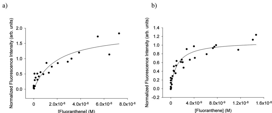
**Fig. 3** Normalized isotherms for (a) fluoranthene in freshwater and (b) fluoranthene in 6 mM octanol from all successful experiments. The fits shown are those for all of the normalized isotherms combined. The correlation coefficients and  $b$  values are: (a)  $b = (1.97 \pm 0.70) \times 10^{-8}$ ,  $r^2 = 0.83$ ; (b)  $b = (1.12 \pm 0.23) \times 10^{-9}$ ,  $r^2 = 0.90$ .
