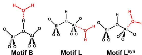
Fig. 1 Interaction motifs for water adsorption on bridging Si–O(H)··AlO<sub>3</sub> groups: Brønsted approach forming an H-bond (motif B) or Lewis-type approach (motifs L or L<sup>syn</sup>).
