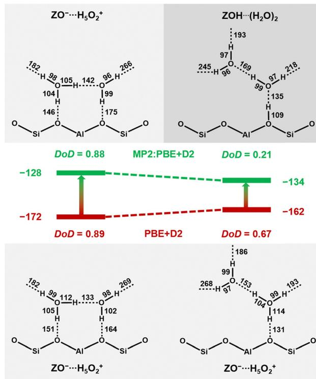
Fig. 8 Ion-pair complex,  $\text{ZO}^- \cdots \text{H}_5\text{O}_2^+$ , and neutral complex,  $\text{ZOH} \cdots (\text{H}_2\text{O})_2$ , for adsorption motif BH at T7 as obtained via structure optimisation with PBE+D2 (bottom) and MP2 (top), see Table 2. DoD defined in eqn (1). The middle part shows MP2+ΔCC adsorption energies in  $\text{kJ mol}^{-1}$ .
