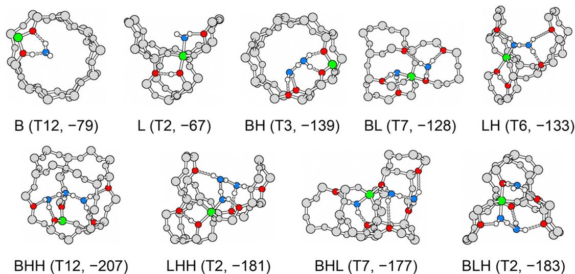
**Fig. 9** Most stable adsorption structures for each interaction motif. Framework position and MP2+ $\Delta\text{CC}$  adsorption energies in  $\text{kJ mol}^{-1}$  in parenthesis. Colour code: aluminium – green, framework oxygen accepting hydrogen bond – red, oxygen in water molecules – blue, framework silicon and oxygen – grey, hydrogen – white.
