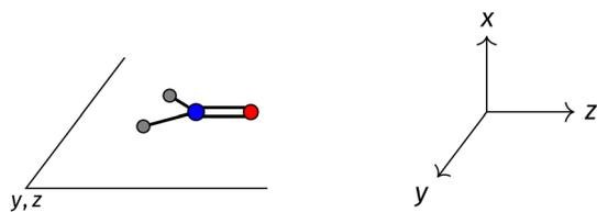
Fig. 1 Geometrical arrangement of  $\text{H}_2\text{CO}$  in all calculations. The molecule lies in the  $yz$ -plane with the C=O bond aligned with the  $z$ -axis. H: grey, C: blue, O: red.
