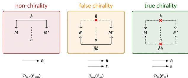
Fig. 7 Barron's classes of chirality and their examples. The systems  $M$  and  $M^*$  are mirror images of each other. In all cases,  $\sigma$  denotes a mirror plane,  $\hat{R}$  a proper rotation, and  $\hat{\theta}$  the time-reversal operation. The magnetic field  $\mathbf{B}$  is an axial time-odd vector, the electric field  $\mathbf{E}$  is a polar time-even vector, and the propagation  $\mathbf{k}$  is a polar time-odd vector.
