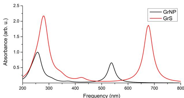
Fig. 4 Theoretical UV absorption spectra of the model graphene lattice both in the optimized (GrNP) and fixed (GrS) geometry forms, computed at TDDFT/ $\omega$ B97X-D3BJ/def2-TZVPP level of theory.
