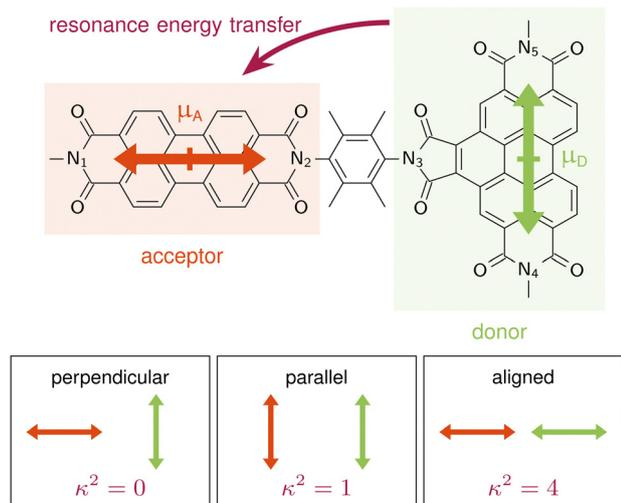
**Fig. 1** Benzoperylene-diimide perylene-diimide dyad (BPDI-PDI), where the TDM of the donor is arranged orthogonally to the TDM of the acceptor and the distance vector. Pictograms on the bottom highlight the orientation factor  $\kappa^2$  according to standard RET theory for distinct TDM conformations.
