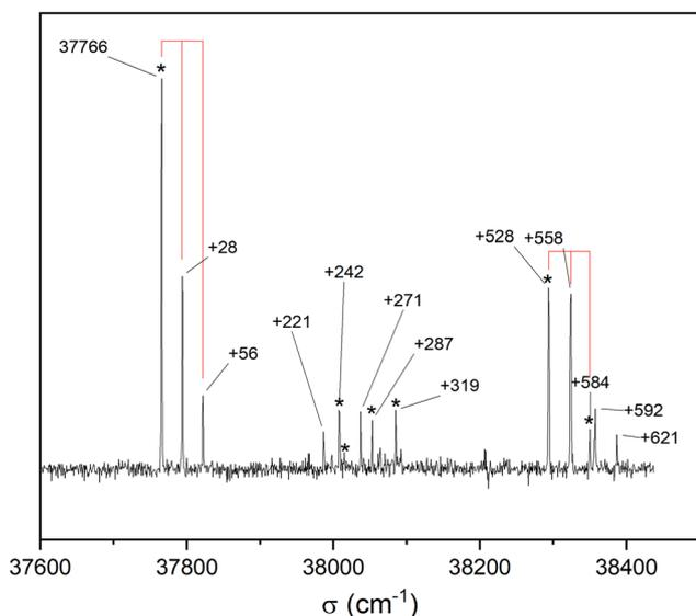
**Fig. 3** REMPI  $S_1 \leftarrow S_0$  electronic spectrum of the *cis*-PCD monomer obtained by monitoring its mass at  $m/z$  192 as a function of the laser wavenumber. The  $28\text{ cm}^{-1}$  progression is materialised by vertical lines. The IR-UV spectra were recorded by setting the probe on the electronic transitions indicated by \*.
