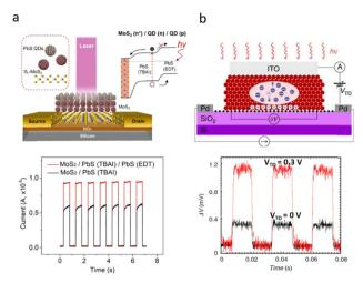
Fig. 8 (a) Device structure of the  $MoS_2/PbS$  QD hybrid phototransistor and its temporal response traces. Reprinted with permission from ref. 97. Copyright 2022, American Chemical Society. (b) Device structure of the hybrid graphene-CQD phototransistor and its temporal response traces. Reprinted with permission from ref. 98. Copyright 2016, Springer Nature Limited.
