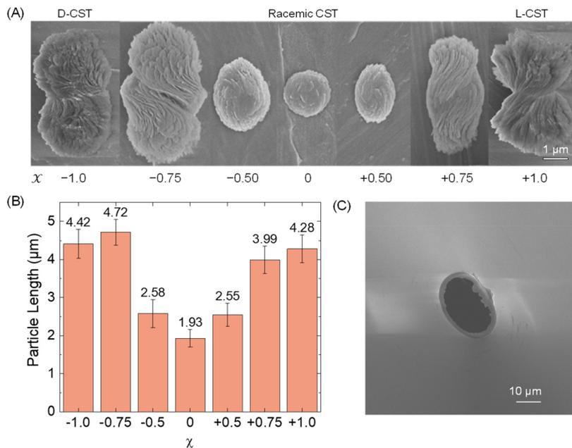
**Fig. 2** (A) SEM images of Cd-CST microcrystals formed at varying enantiomeric excess ( $x$ ).  $x = -1.0$  means 100% D-CST and 0% L-CST, while  $x = 0$  means a racemic mixture of 50% D-CST and 50% L-CST. (B) Particle length distributions of Cd-CST crystals at varying  $x$ . The error bars are the standard deviations of particle lengths after analyzing at least 100 particles. (C) SEM image of a micropipette used in the resistive pulse analysis of Cd-CST crystals.
