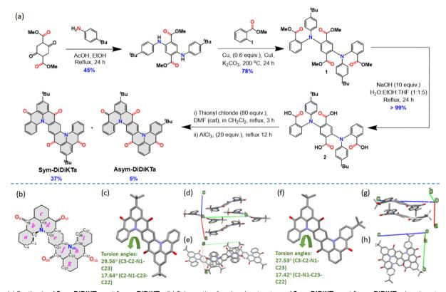
Fig. 2 (a) Synthesis of Sym-DiDiKTa and Asym-DiDiKTa. (b) Schematic of molecular structure of Sym-DiDiKTa and Asym-DiDiKTa showing atom labels (double bonds omitted for clarity). (c and f) View showing Sym-DiDiKTa and Asym-DiDiKTa in the crystal structure (diagonal view). (d and g) Side view of the packing diagram of Sym-DiDiKTa and Asym-DiDiKTa. (e and h) Top view of the packing diagram of Sym-DiDiKTa and Asym-DiDiKTa
