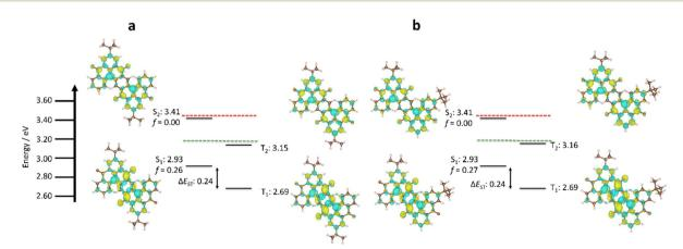
Fig. 3 Difference density picture and excited state energies of Sym-DiDiKTa (a) and Asym-DiDiKTa (b) calculated at SCS-CC2/cc-pVDZ, where red and green lines indicate  $S_1$  and  $T_1$  energies respectively of **DiKTa**, (isovalue = 0.001).
