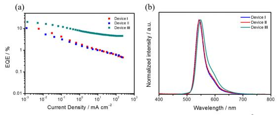
Fig. 6 (a) EQE versus current density curves of Devices I-III. (b) Electroluminescence spectra of Devices I-III at 500 cd m<sup>-2</sup>.
