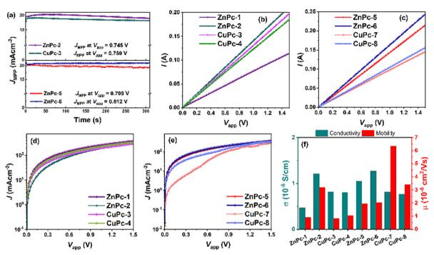
Fig. 7 (a) Steady-state photocurrent density for the continuous illumination at the maximum power point (MPP) for the devices in symmetric and asymmetric MPcs as HTLs, I-V curves for the conductivity measurement in the configuration of FTO/MPc/Ag for (b) symmetric MPcs and, (c) asymmetric MPcs, J-V curves for the hole mobility measurements in the configuration of FTO/PEDOT: PSS/MPc/Aq for (d) symmetric MPcs, and (e) asymmetric MPcs and (f) conductivity and mobility of each MPc summary
