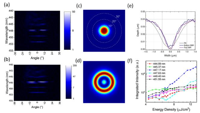
Fig. 5 Defect microcavity dispersion (a) below threshold (7.7  $\mu$ J cm<sup>-2</sup>) (b) above threshold (12.0  $\mu$ J cm<sup>-2</sup>), Numerical simulation of the far-field projection for cylindrical defect (c) lowest energy mode (d) lasing mode (e) Defect profile for each layer of the microcavity, measured with AFM (f) Integrated intensity extracted from the Fourier imaging dispersion as a function energy density for each emitting mode with lasing coming from 447.17 nm.
