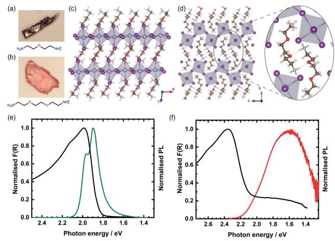
Fig. 1 (a) OBESnI<sub>4</sub> and (b) EDBESnI<sub>4</sub> images of mm-sized single crystals. Crystal structure of (c) OBESnI<sub>4</sub> and (d) EDBESnI<sub>4</sub>, where grey atoms are Sn, purple are I, blue are N, brown are C, red are O, and white are H. The inset highlights the formed hydrogen bonds. Kubelka-Munk transformed diffuse reflectance and photoluminescence spectra of (e) OBESnl<sub>4</sub> and (f) EDBESnl<sub>4</sub>
