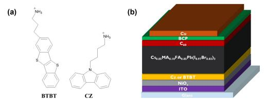
Fig. 1 (a) Molecular structure of BTBT and Cz. (b) Perovskite solar cell stack depiction. The control sample does not contain any modification between NiOx and the perovskite laver
