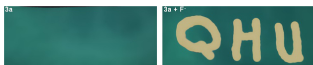
Fig. 5 The 3a based film sensors for fluoride anions under UV irradiation ( \lambda_{\text{ex}} = 365 nm).
