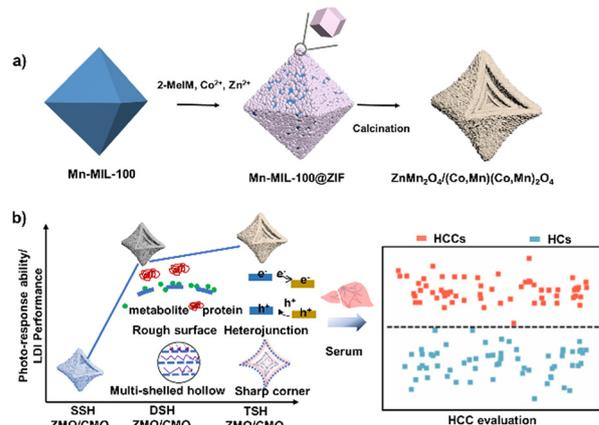
**Scheme 1** Schematic illustration of the (a) synthetic route to triple-shelled  $\text{ZnMn}_2\text{O}_4/(\text{Co}, \text{Mn})(\text{Co}, \text{Mn})_2\text{O}_4$  (TSH ZMO/CMO) and (b) LDI-MS extraction of serum metabolic fingerprints by TSH ZMO/CMO with specific physical effects for evaluation of hepatocellular carcinoma (HCC).
