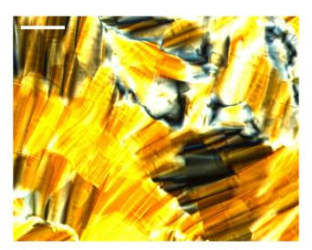
Fig. 9 Cross polarised optical microscopy image of 30 wt% phytantriol in a solvent mixture containing 70 wt% ChCl:U and 30 wt% water at °C. Birefringent texture is consistent with a hexagonal phase. Scale bar is 100 µm.
