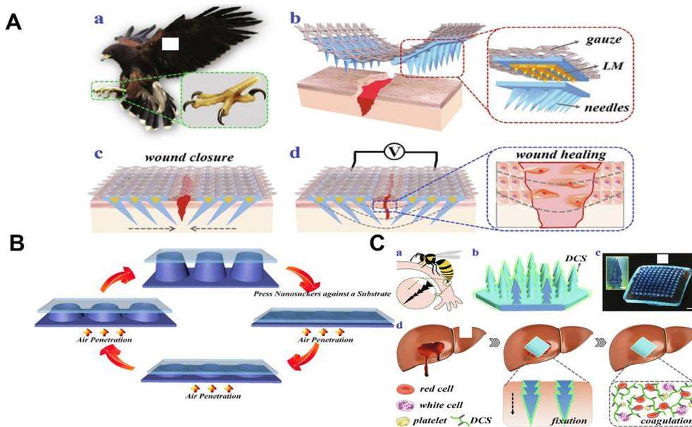
Fig. 5 (A) Schematic illustration of the claw-inspired microneedle patch with liquid metal encapsulation and its wound healing application.<sup>86</sup> Copyright 2021 Elsevier. (B) Schematic diagram of the working principle of the microneedle patch and the equipment process.<sup>91</sup> Copyright 2017 American Chemical Society. (C) Schematic diagram of the preparation of a hemostatic and bionic pagoda microneedle patch.<sup>99</sup> Copyright 2021 Elsevier.
